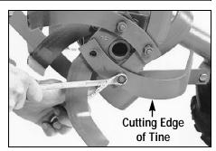
Figure 5-6: Removing single tine.
